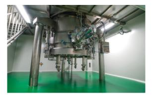
Temperature range: -100° C ~ +300° C Pressure: Max. 10 MPa (Fluorination) Max. 4 MPa (Hydrogenation)
