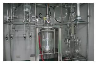
50 walk-in hoods). Dalian's kilo lab facilities include 50-L and 20-L reactors, thin-film evaporator, fractional distillation equipment, and rotary evaporator. This allows us to rapidly scale up lab process to produce advanced intermediates in kilogram scale.
